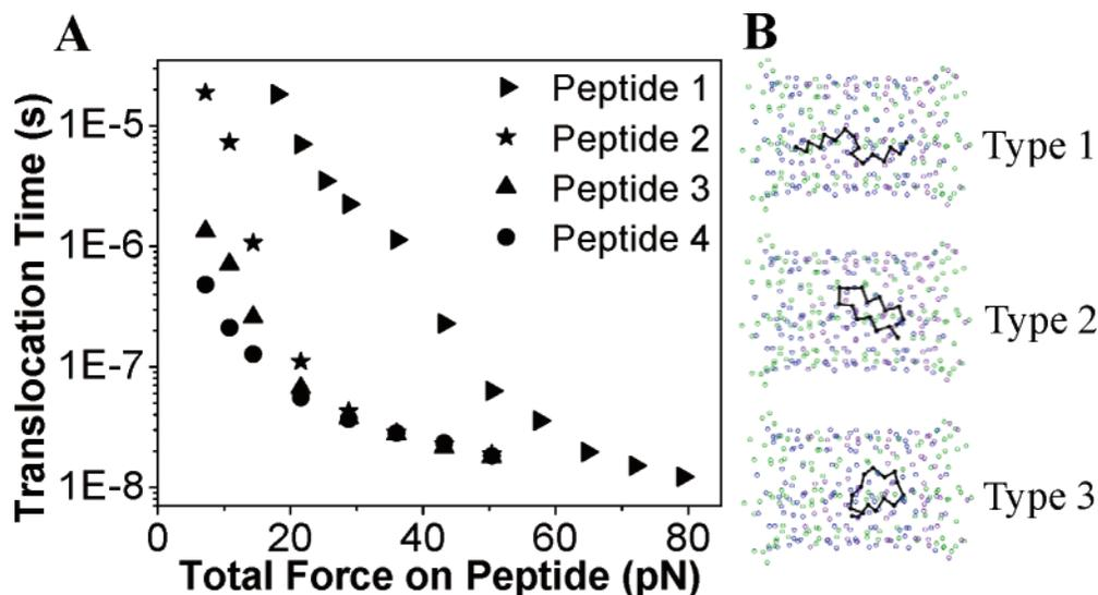
**Figure 3.** (A) Computed mean translocation time as a function of the total force on the  $\beta$ -hairpin. (B) Typical conformations of the peptide inside the  $\beta$ -barrel part of the  $\alpha$ HL pore corresponding to three types of observed translocation trajectories. See the Supporting Information for the animations of the entire trajectories. Only the positions of the  $C_{\alpha}$  atoms are shown in the pore structure.
