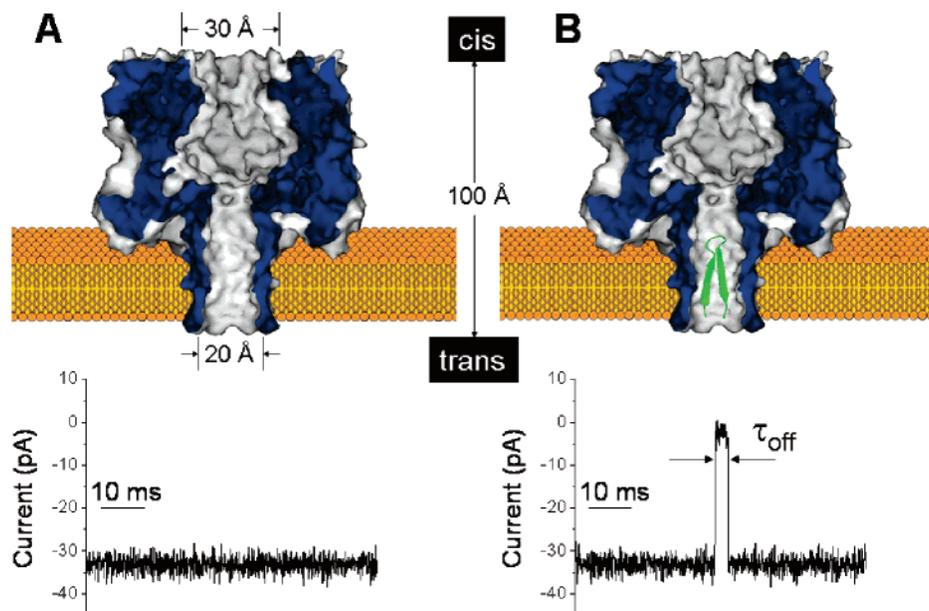
**Figure 1.** Interaction of  $\beta$ -hairpin peptides with an  $\alpha$ HL pore: (A)  $\alpha$ HL forms a channel that remains open for long periods. (B) The translocation of a  $\beta$ -hairpin peptide through an  $\alpha$ HL pore produces a transient current blockade.
